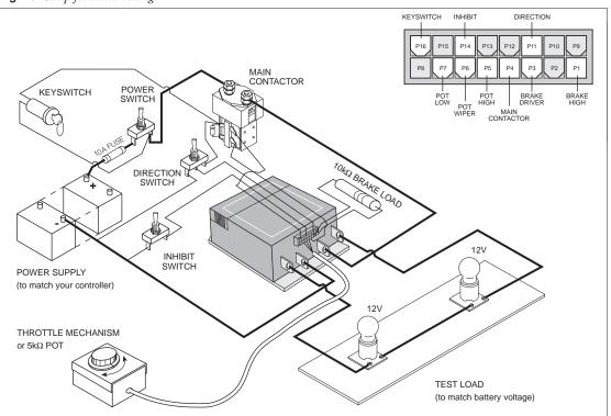
Fig. 13 Setup for bench testing.
