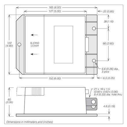
Fig. 2 Mounting dimensions for the Curtis PMC 1213 controller.
