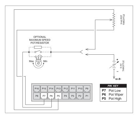
**Fig. 7** Wiring for maximum speed limiting potentiometer/resistor.
